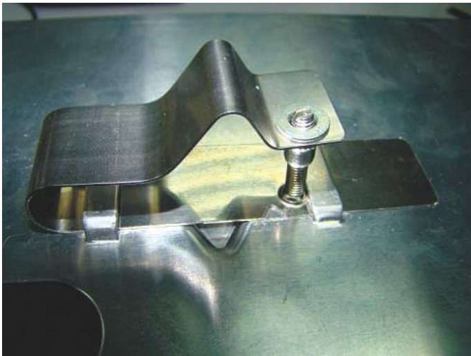
Fig. 25 The screw hole of adjustment clamp contact with the indicated profile of lung plate punch as much as possible.
