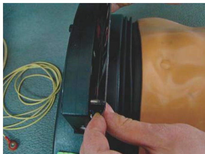
Fig. 4 Disassemble both 2 slotted pins, and then take the front scale plate out.
