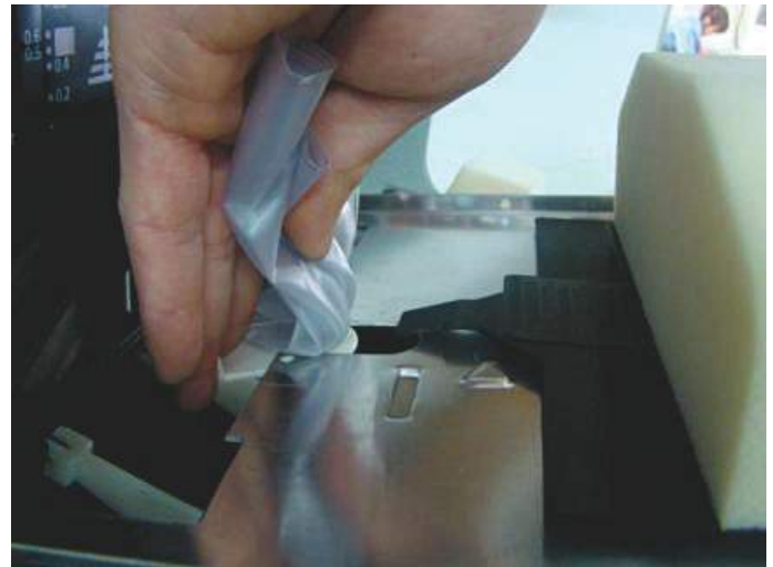
Fig. 28 Fold the stomach bag in case it is damaged by the sharp edge of lung plate. Mount the stomach bag to lung plate kit.
