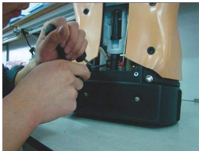
Fig. 38 Remove the Battery compartment. Adjust the screw in the adjustment clamp to zero the compression indicator.
