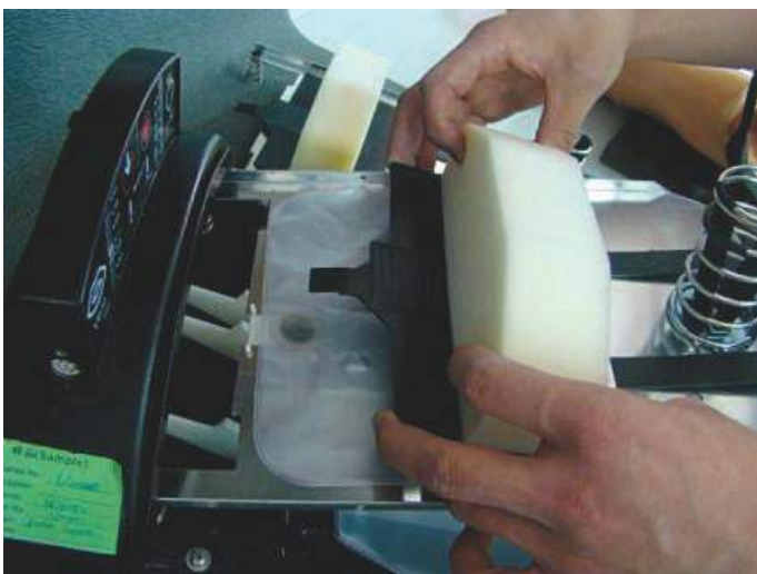
Fig. 29 Unfold the stomach bag and make sure it is flat on the lung plate.
