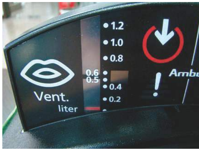
Fig. 40 The indicator shows "0" litre and starts moving as soon as ventilation is done. When finally adjusted mount the battery compartment.
