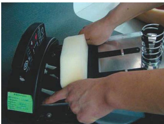
Fig. 21 Press two springs at the end of the lung plate and pull the lung plate out at the same moment.
