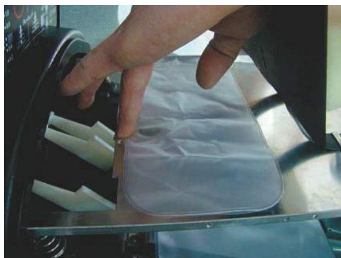
Fig. 22 Push the stomach bag on the lung plate and disassemble it.
