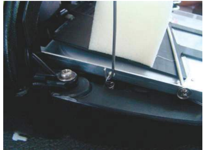
Fig. 34 Mount new side spring in the lung plate.
