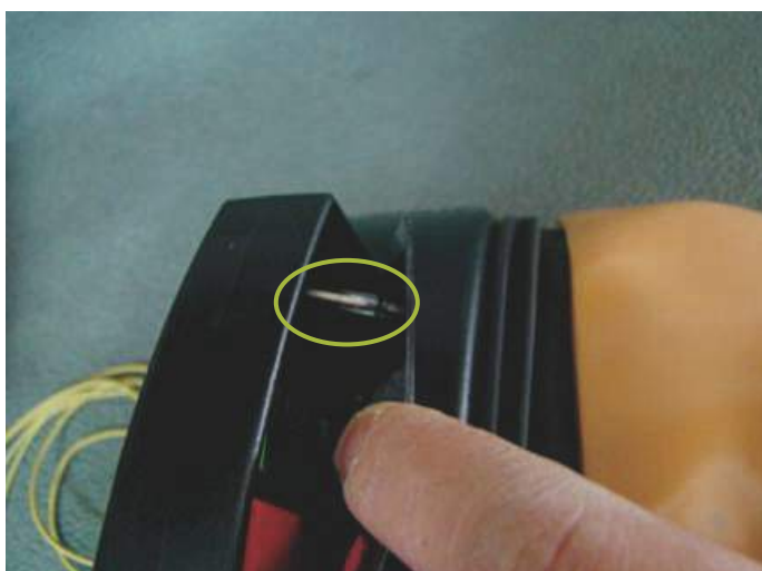
Fig. 3 Force the slotted pin to lock back and front scale plate to be separated.
