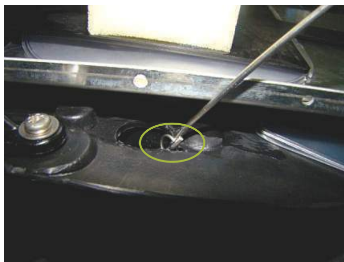
Fig. 18 Disassemble the side spring on the lung plate. Replace the old side spring with new spring.
