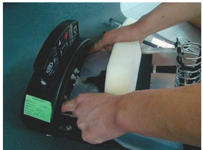
Fig. 30 Press two springs at the end of the lung plate and push the lung plate into the belt pad.
