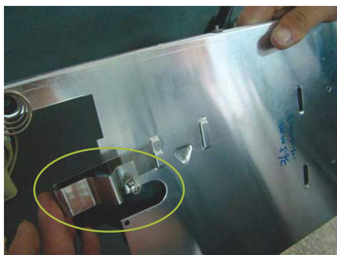
Fig. 24 If not already mounted, mount the new adjust clamp unit to new lung plate.
