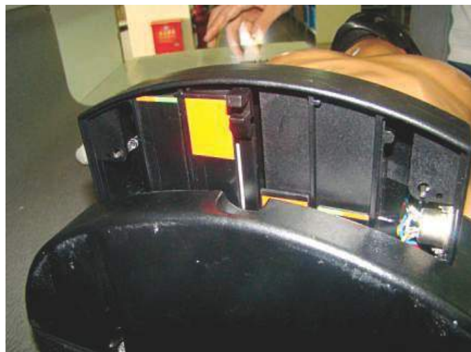
Fig. 8 Finish the new front plate assembly. Check if the slotted pins are in position.
