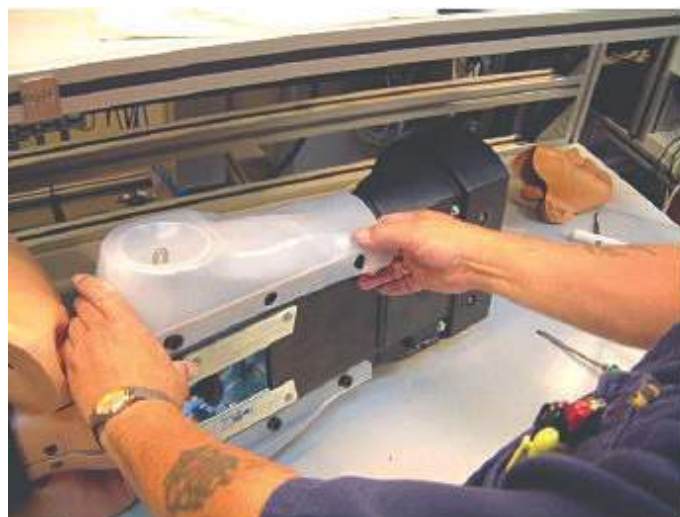
Fig. 14 Remove by lifting each part of the chest. During removal, treat as gently as possible.
